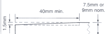
Fig. 7 SITE-GROUND RECESSED-EDGE DETAIL
